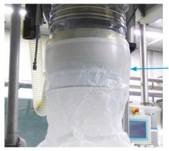
When inflated, the outer Seeflex layer will securely hold the bag neck up and open for clean, efficient filling.
