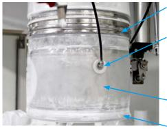
BFM® spigot welded to outlet pipe/chute
