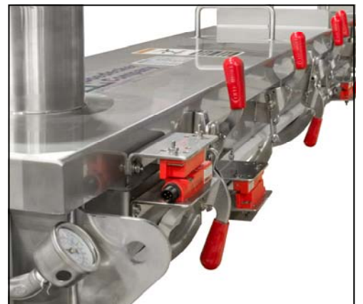
Close-up of clamps
